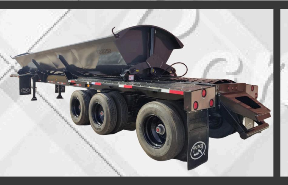
Instantaneous air exhaust-height control valve Any color combinations for paint job (10) 24.5 x 8.5 steel wheels with radial tires. Options:
